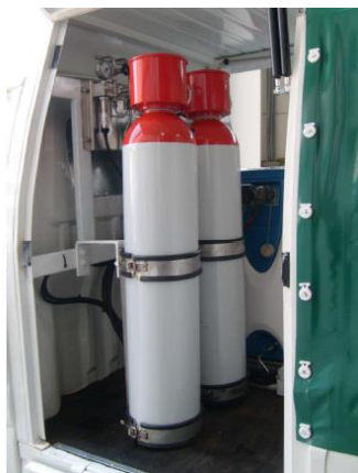
Picture 5: H2 Pressure cylinders in the vehicle
